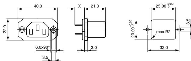
Lötanschlüsse 6.3 x 0.8 mm: x = 11.2 mm
